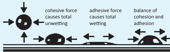
Antispread reduces the surface tension of the solid as far as silicon oil can't spread any more.
